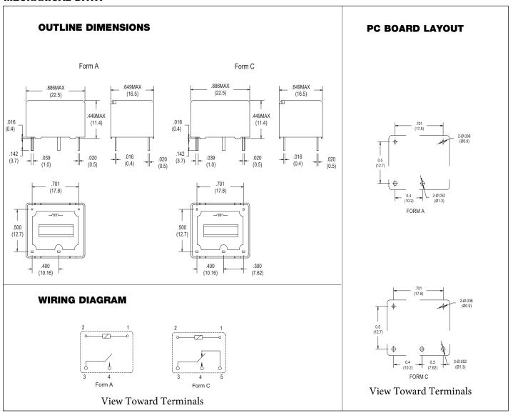
Dimensions in inch with millimeters in brackets below, Tolerance: ±0.010"
